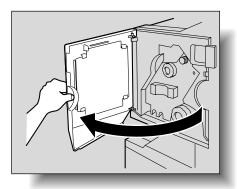
2 Turn misfeed-clearing dial ① clockwise until the removal indicator is completely blue.
